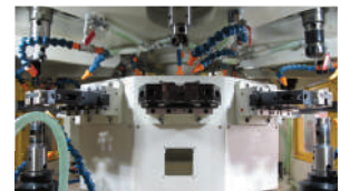
High-strength, high-precision synchronizing chuck for minimal blank OD change and symmetry of output.
