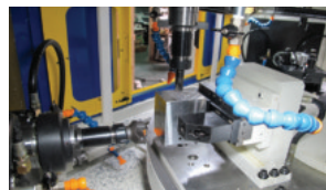
Servo-slide simultaneously tri-directional (upper, middle and lower) processing
