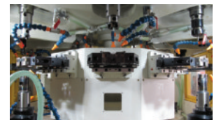
High-strength, high-precision synchronizing chuck for minimal blank OD change and symmetry of output.
